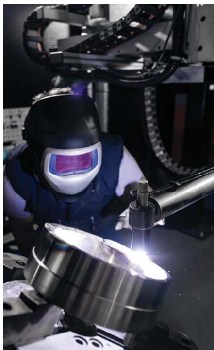
Body seats being welded.
