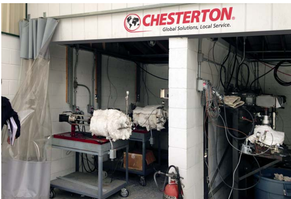
Fully automated test lab – packing and valve testing.
