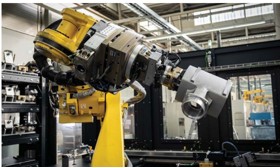
AUMA’s latest investment in manufacturing and testing technology is a fully automated test bench to burst-test the housings of explosion-proof actuators. A robot places the housing parts in a pressure chamber where they are subjected to a pressure of 60 bar.
