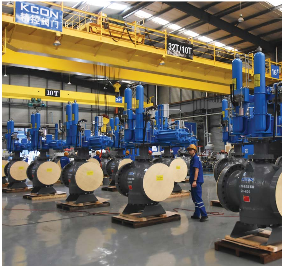
KCON has supplied numerous pressure-balanced plug valves in sizes up to 24" and pressure classes up to #900 to the prestigious
