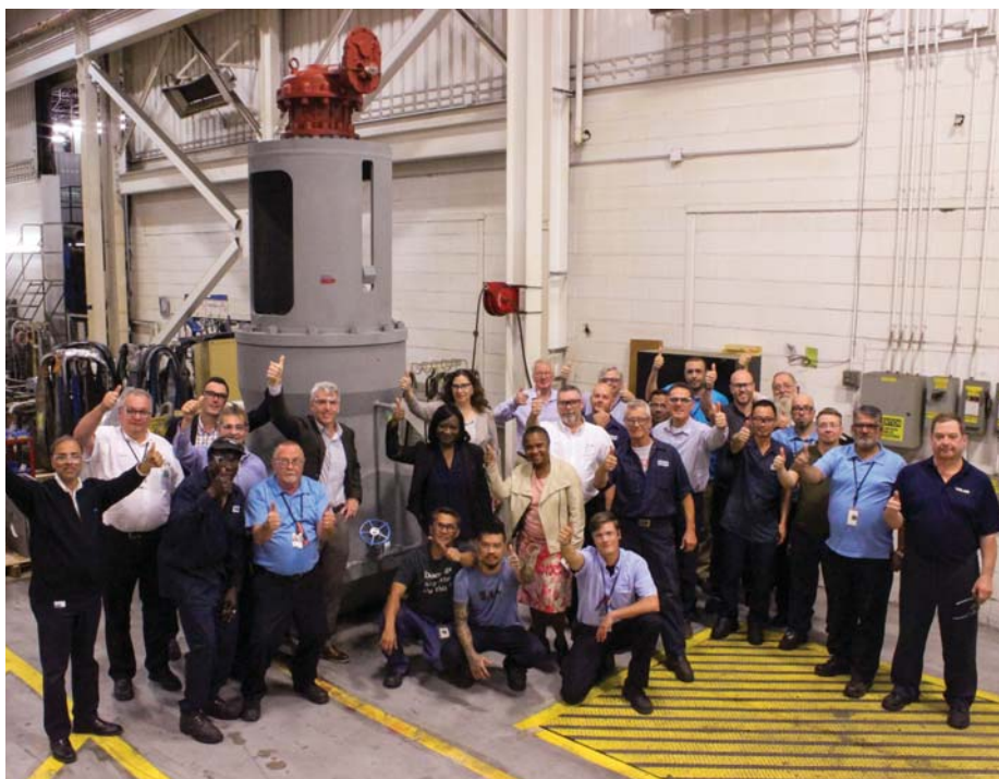
Weighing 36,000 lbs, Velan's first ever 34" Class 1500 forged pressure seal parallel slide valve, part of an order for two 24" and two 34" valves for main steam isolation in an olefins plant in Southern Texas. Although the designs were new and posed many technical challenges, the valve was delivered on-time under tight deadlines, thanks to VPM governance.
