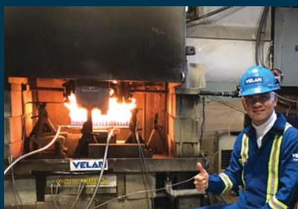
Duke Tran, witnessing the fire testing of five Velan valves including ball and triple-offset valves, resulting in a 100% pass rate.
