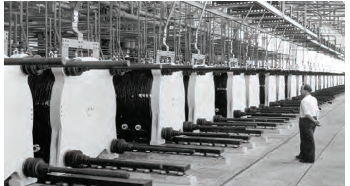
Electrolysis in Glomfjord-site of Yara. The company employed this technology until it was outcompeted by SMR.
