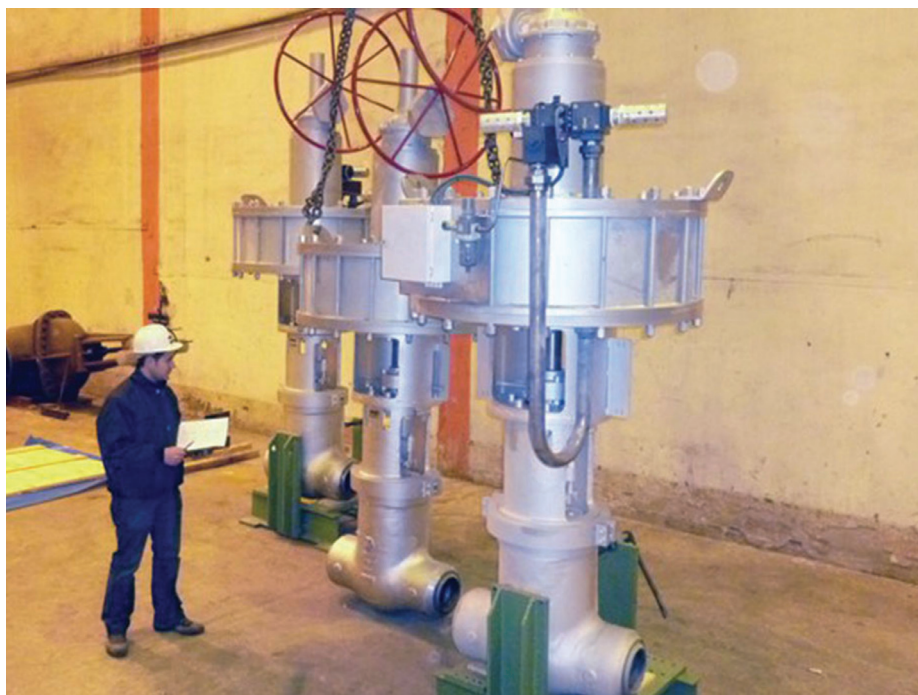
Figure 2 – Valves with large actuators may need additional bracing. Image courtesy of Babcock Valves.
