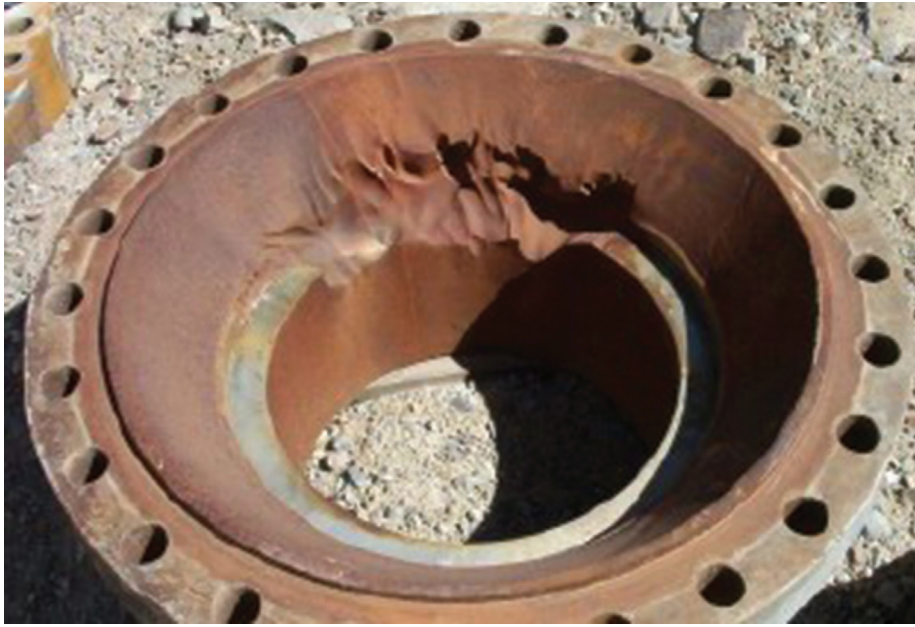
Figure 3 - Damage most likely provoked by erosion in a ball valve used for throttling. Image courtesy of Copeland Ball Valves.
