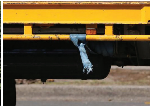
Figure 1 – A jet engine worth around $45 million new fell off a truck. Above, the likely cause, a cheap strap.
