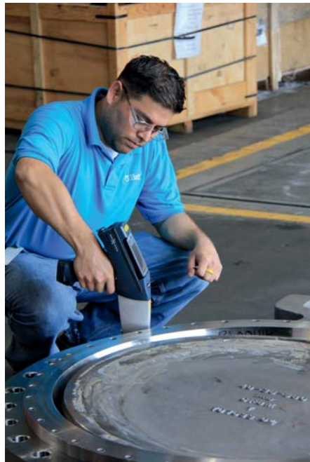
Inspector performing PMI testing.
