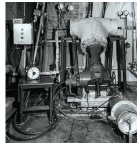
1960s Velan designed tested the 5-16" (125-400 mm) forged parallel slide gate valves for the USS Nimitz Aircraft Carrier, which was the first of nine nuclear-powered Nimitz Class Aircraft Carriers to be built.
