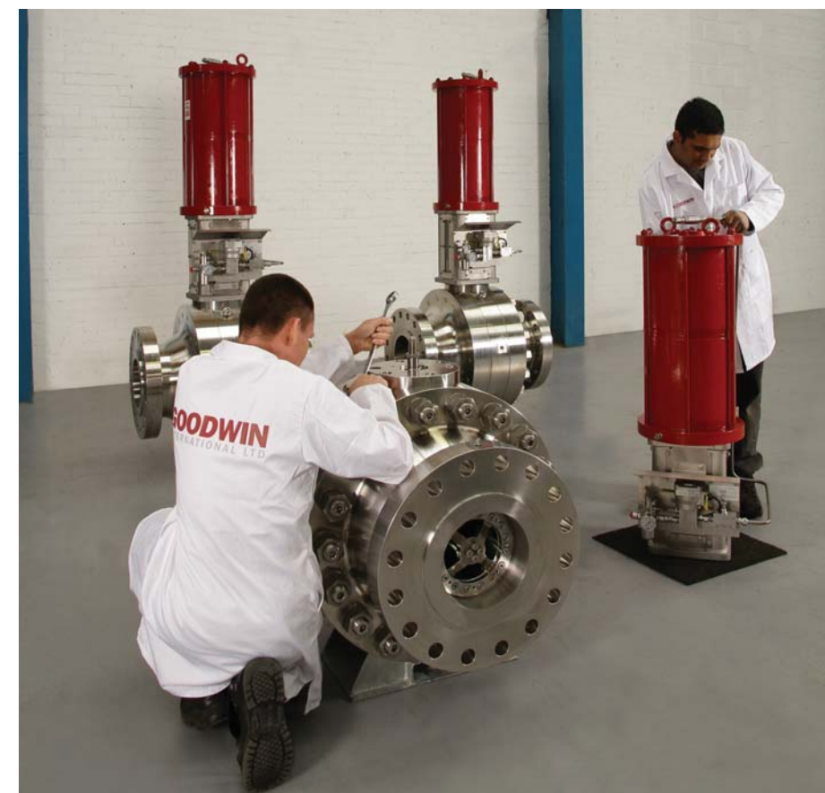
The assembly of the control valve. Goodwin has been able to draw on a highly skilled workforce, many of whom were trained in-house.
