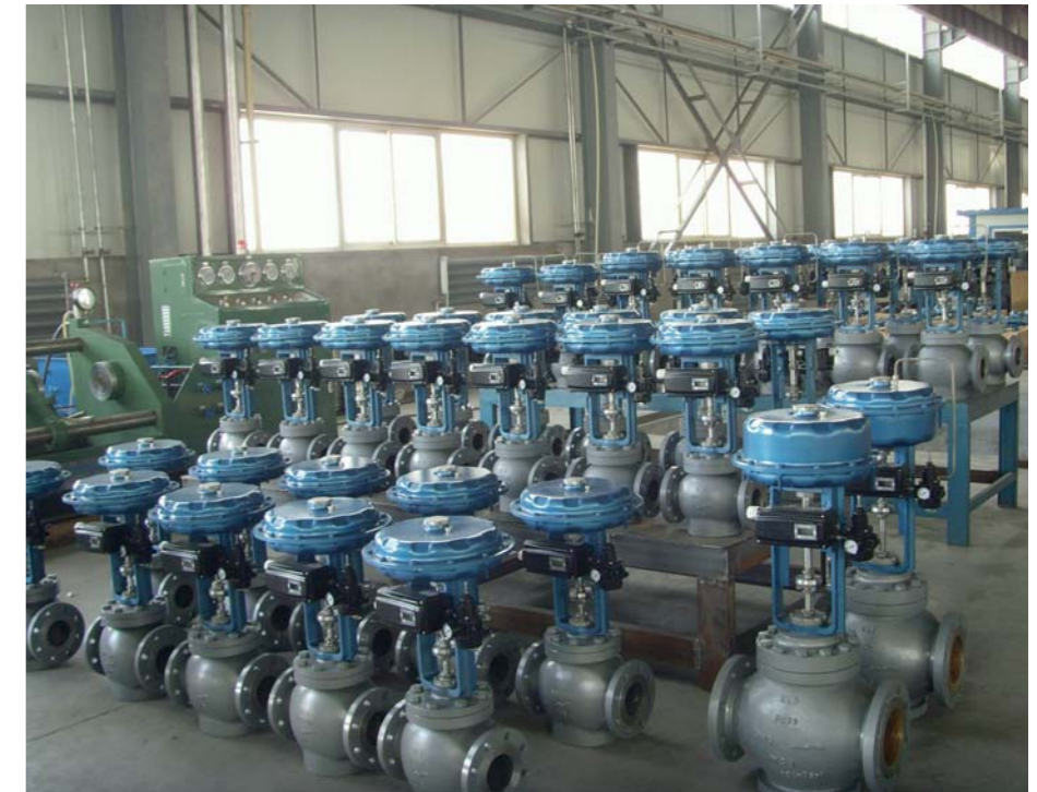
The YT-3300. At the heart of this range of SMART positioners, YTC utilises torque motor/flapper nozzle technology for converting the electrical input signal to a pneumatic output signal.
