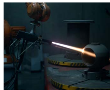
High velocity oxygen fuel spraying.
