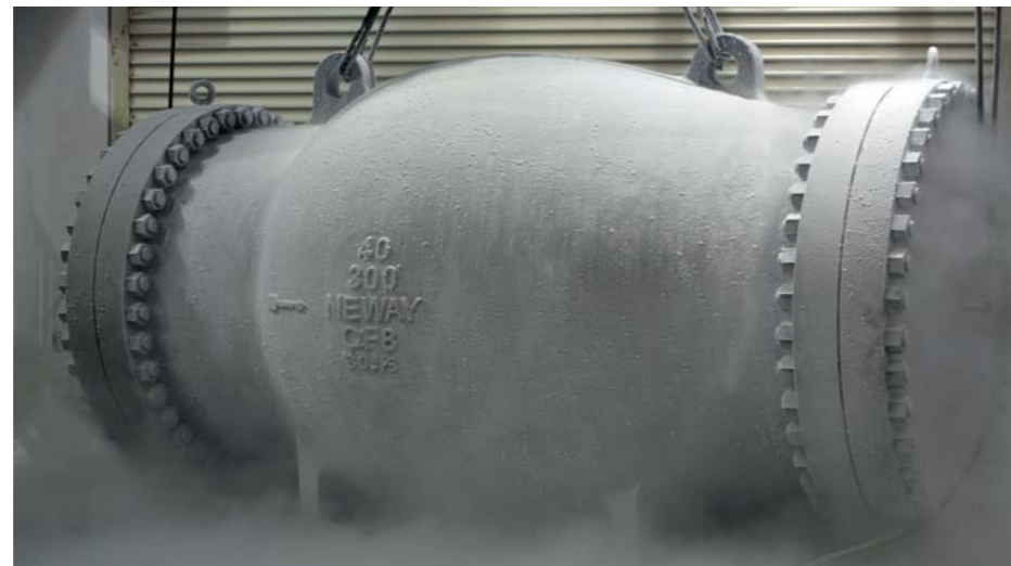
In-house cryogenic testing of axial flow check valve.
