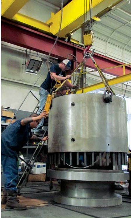
Assembling 36” 600 SCV Trunnion Mounted Ball Valve.
