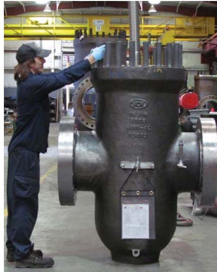
Assembly of 16-3/4" – 5000 PSI SCV API 6A Thru Conduit Gate Valve (Expanding Gate Design).
