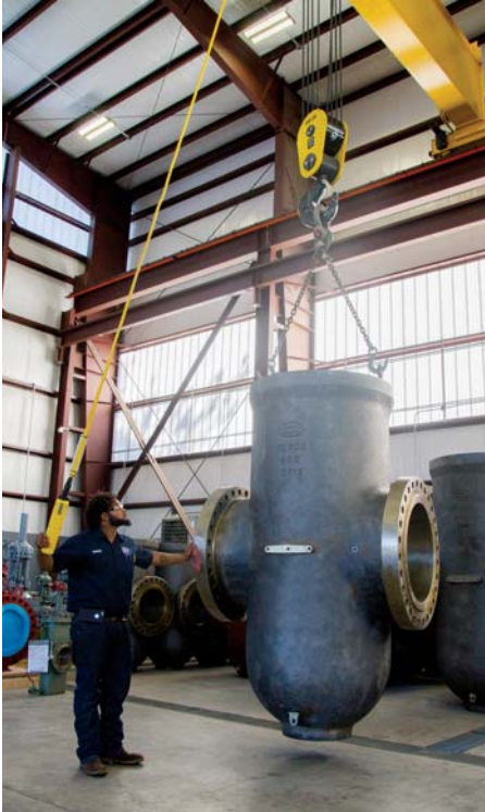
Moving 30” 600 Thru Conduit casting into position for assembly.
