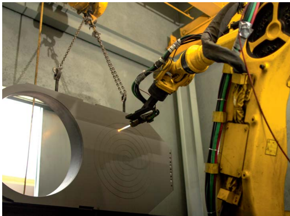
The company assures that their valve quality is further assured with the aid of in-house test facilities including X-Ray source Iridium 192, impact, tensile, hardness, adhesion test equipment, measuring coordinate table and their own HVOF process for applications of tungsten carbide or chromium carbide coatings, among others. Seen here the HVOF process.
