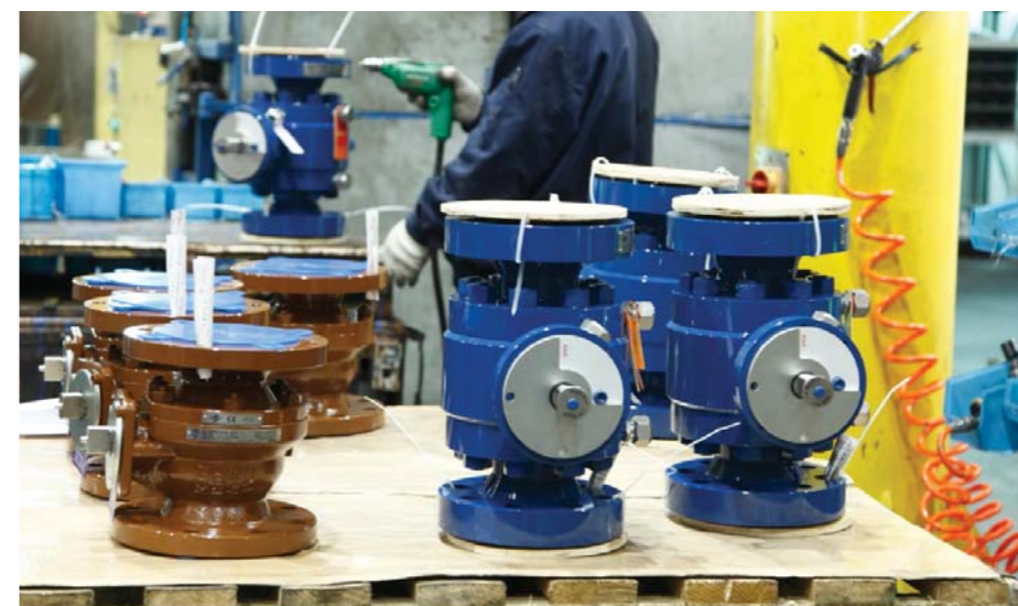
CIRCOR Energy's KF Valves floating flanged ball valve (Series F) and trunnion mounted ball valve (Series P3) being prepared for shipment.
