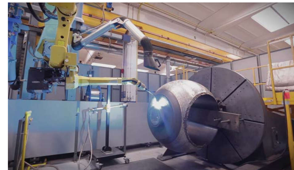
Weld overlay procedure on a large ball for an engineered ball valve in CIRCOR Energy's Milan, Italy facility.
