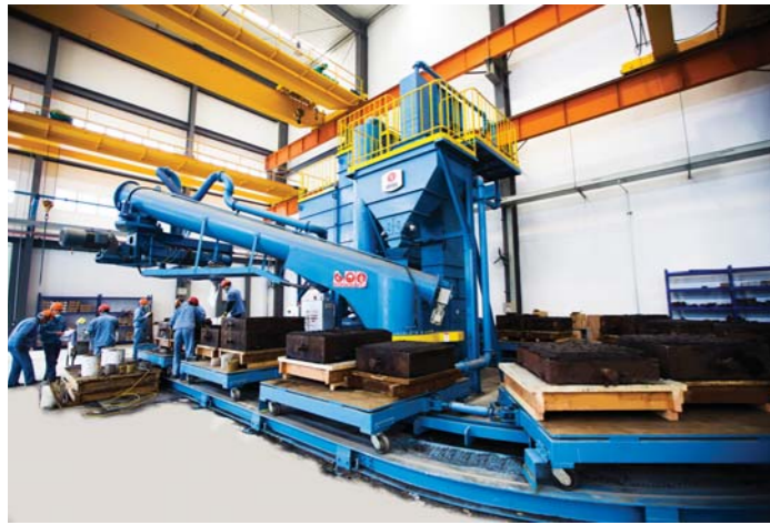
Fig. 3. The mixer and semi-automatic molding line in new foundry.
