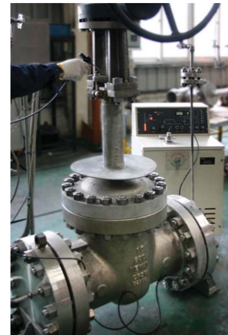
Low emission sniff testing of Neway gate valve
