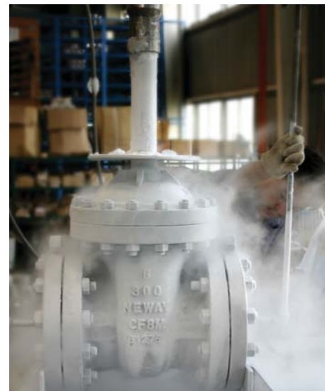
In-house cryogenic testing of Neway gate valve
