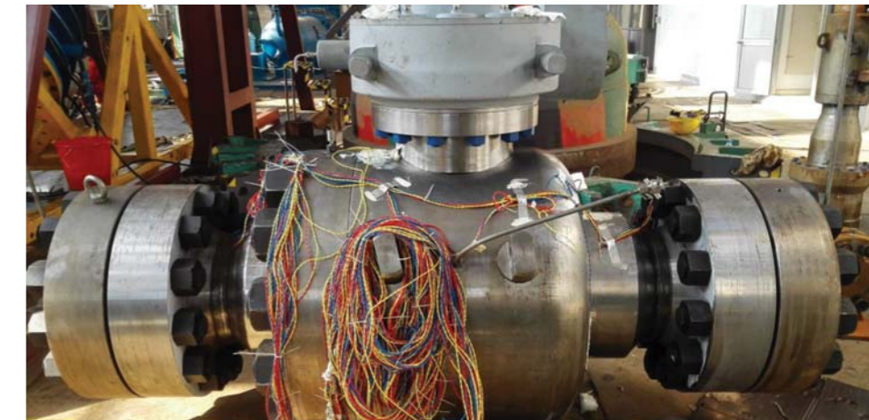
Subsea ball valve being prepped for hyperbaric chamber testing
