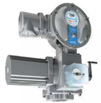
Specialised technology including an integrated frequency converter enables SIPOS to provide actuators with variable speed control. Soft-starts and finishes are facilitated, avoiding problems such as water hammer.
