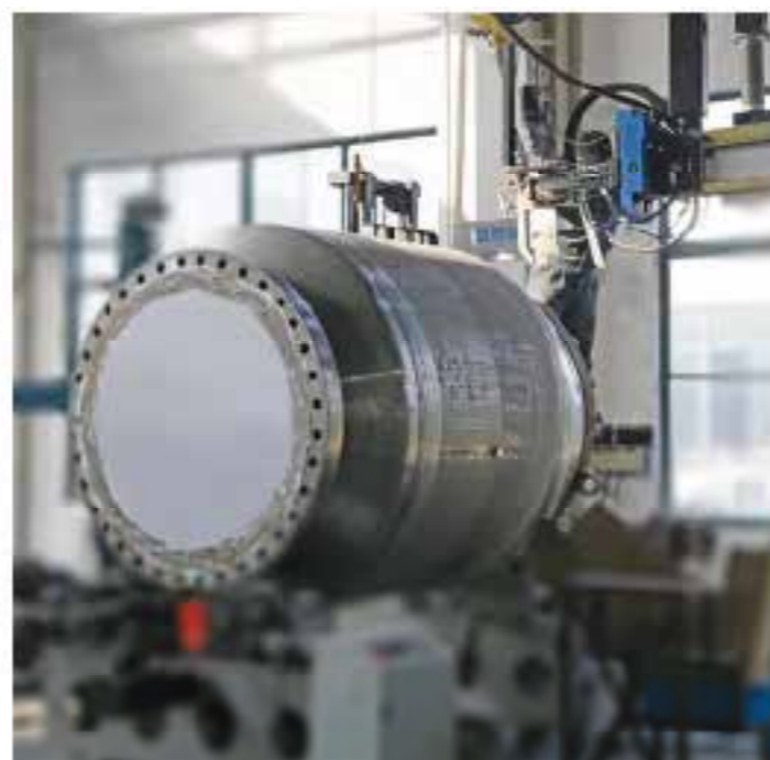
42 inch, fully welded ball valve.
