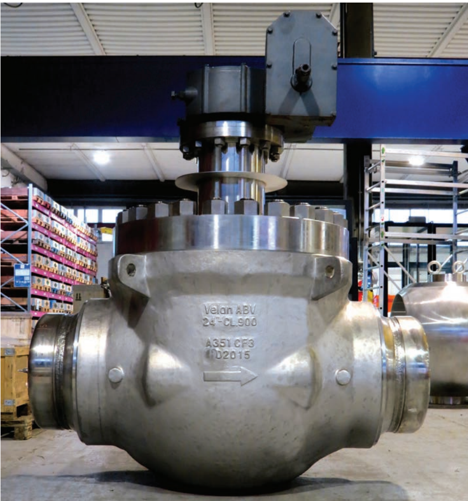
Part of a package of cryogenic side-entry and top-entry ball valves from 6-24", ASME 900 class, temperatures to -196 °C, destined for a project in Asia.
