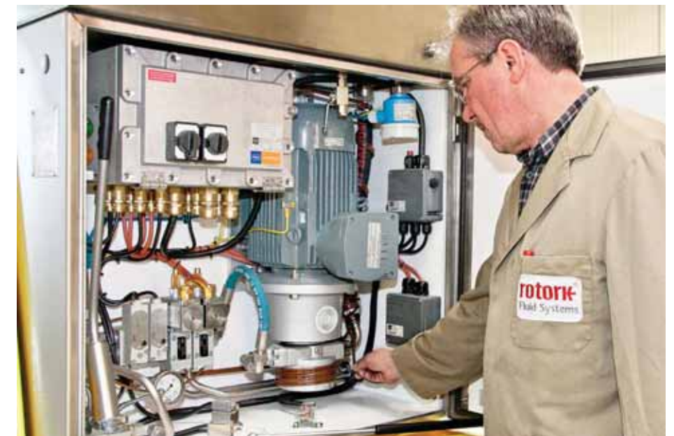
Control cabinets for actuators destined for the Russian territories are amongst those designed and manufactured at the Melle factory.
