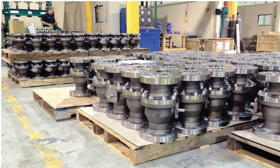
ViNtrol Valves staged for Hydro Test.
