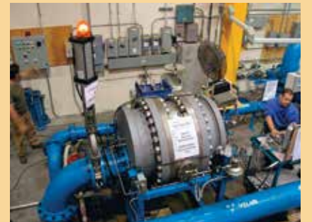
Qualification testing of a 34" titanium triple-offset butterfly valve in Velan's R&D lab. The valve had no leakage over the 10,000 cycle test.
