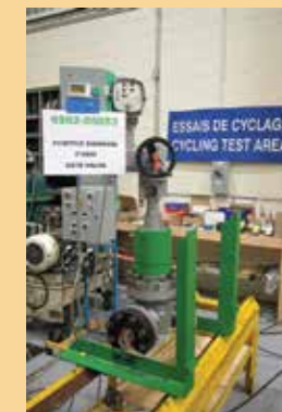
Cycle testing for fugitive emissions today targets 600, 900, and 1500 class valves.
