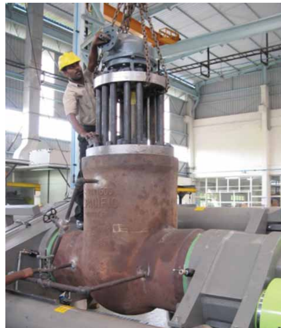
24" Class 1500 Gate valve on a test unit HC2000-CR
