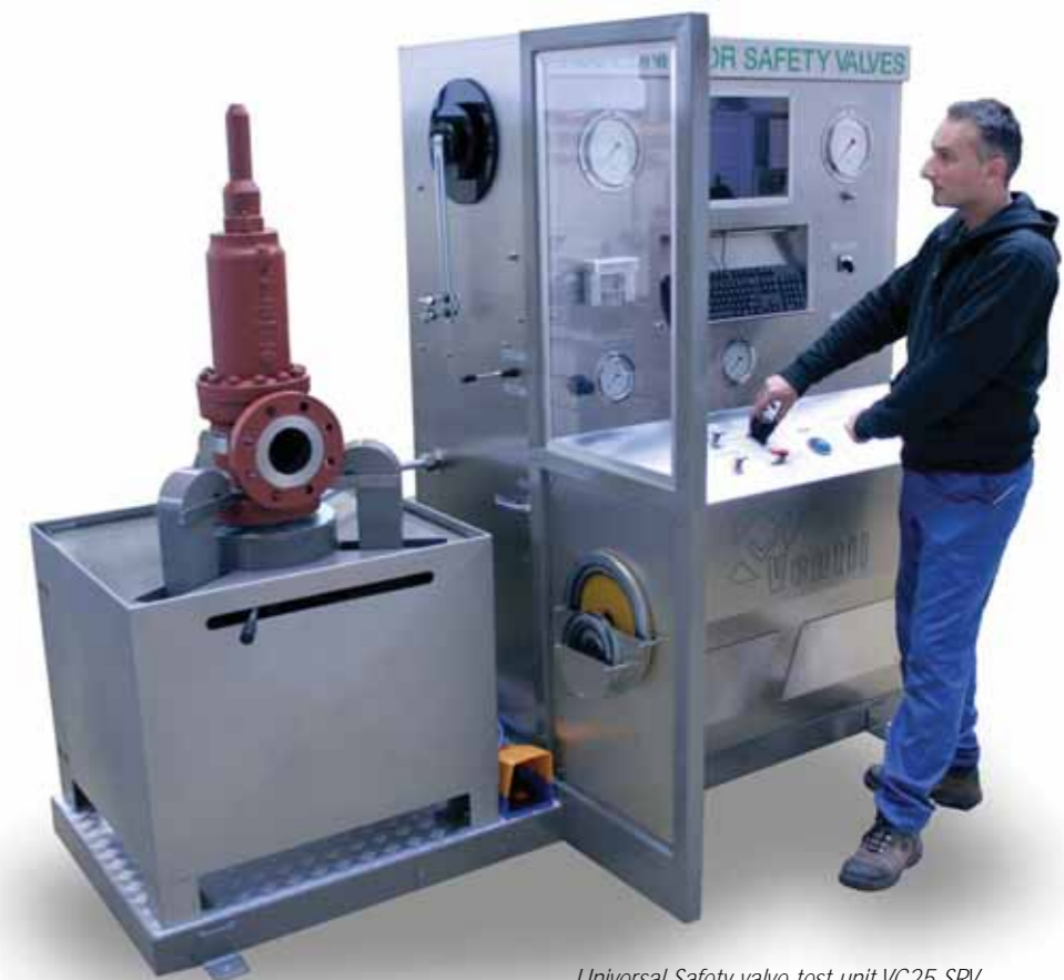
Universal Safety valve test unit VC25-SRV
