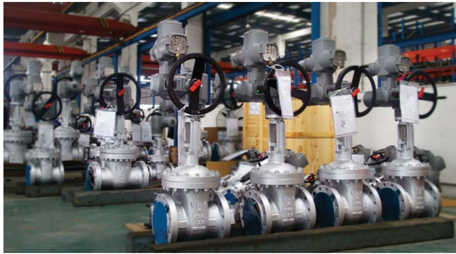
AUMA electrical actuated gate valves.
