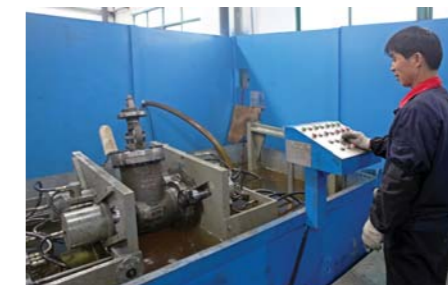
High pressure air shell test.
