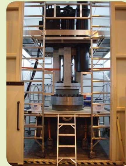
Main steam isolation valve ready for pressure testing.
