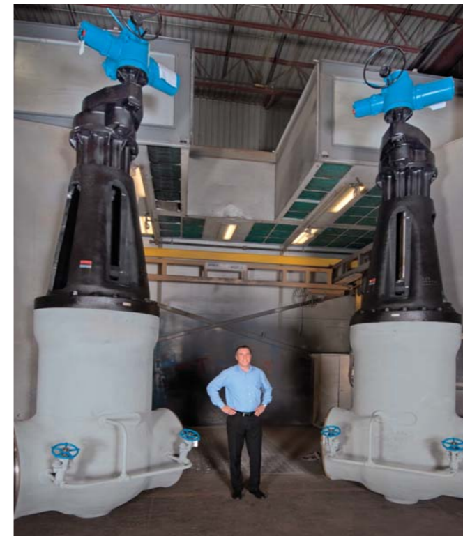
Joe Calabrese, Velan's Director of Sales for East Asia, with two large Velan 36" Class 900 pressure seal valves for a power plant in China.
