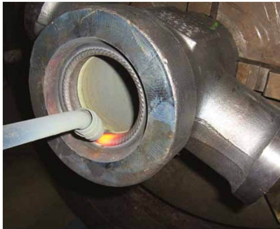
Featured: Alloy 625 wetted surface weld cladding in process.
