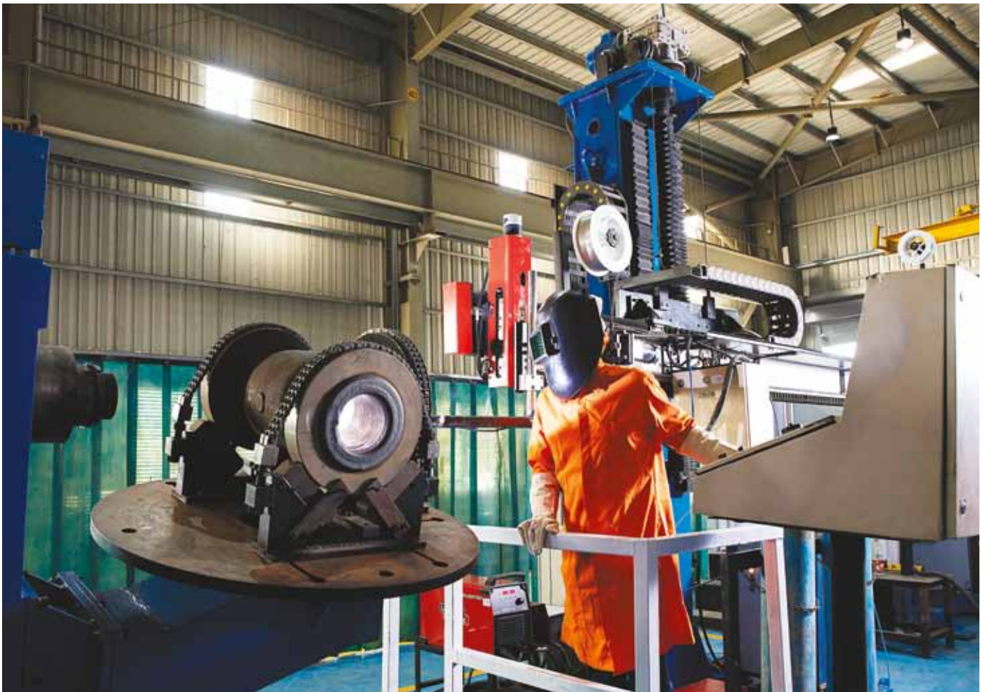
Cladding using Automated Welding Machine
