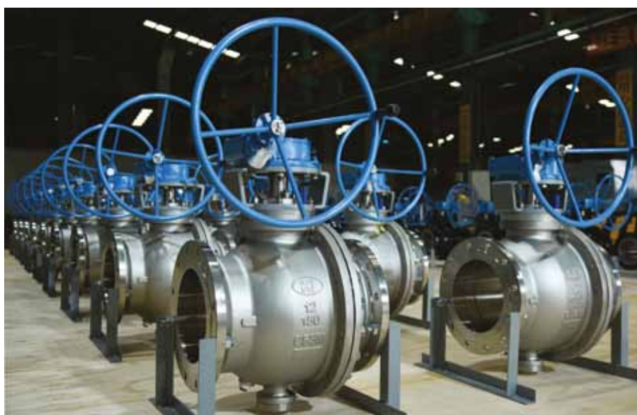
Trunnion ball valve (ANSI & DIN pressure; size range from 3" to 24").
