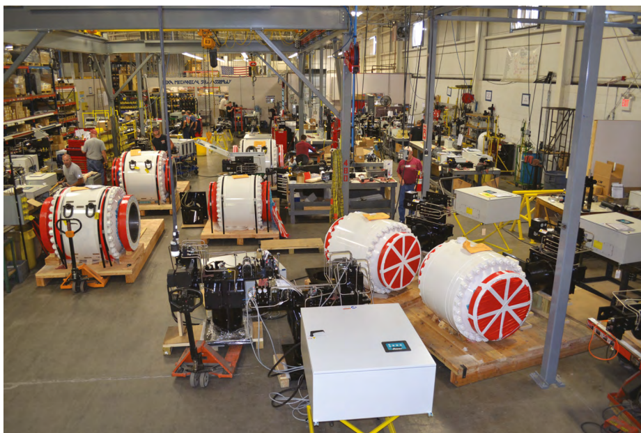
Main factory doing mount-cal-testing on large modulating ball valves.
