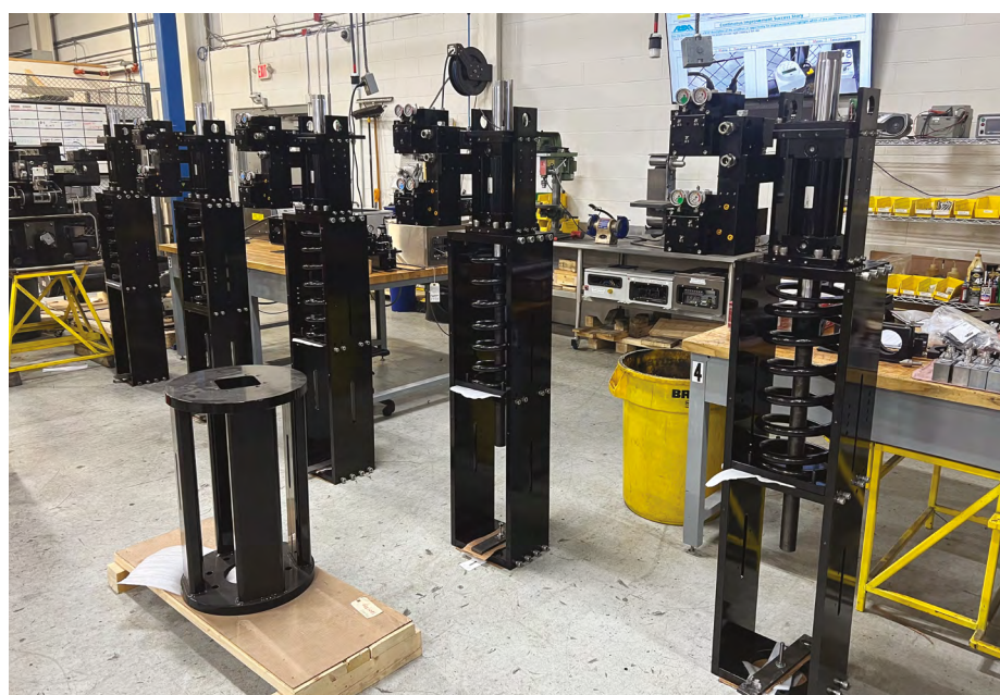
Compressor anti-surge actuators to replace pneumatics at a refinery in Saudi Arabia.
