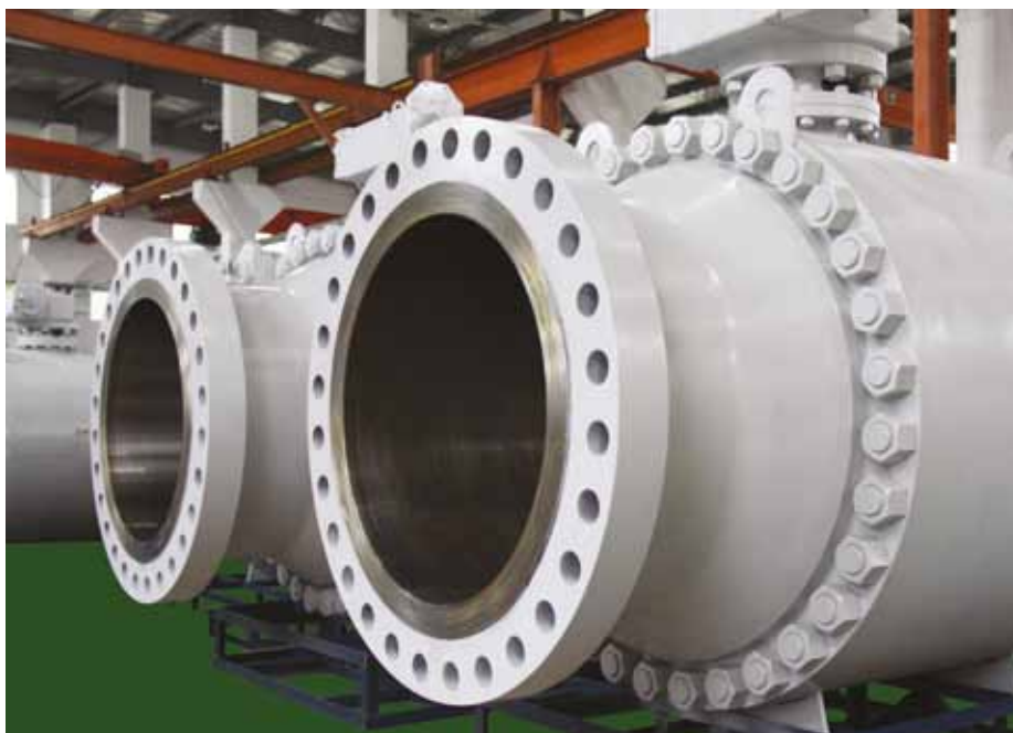
This special high-strength ball valve on a pipeline is FEA verified.
