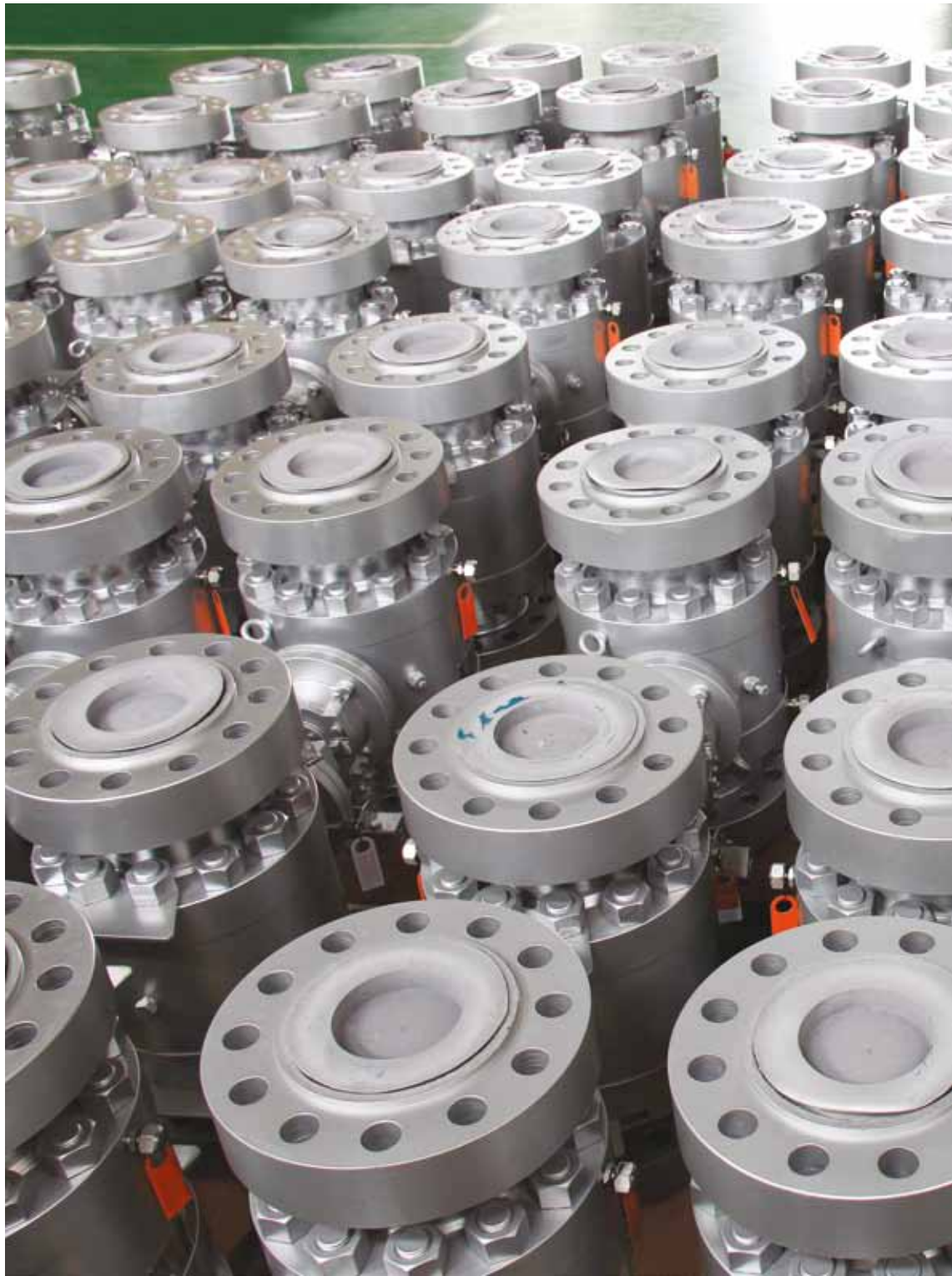
6" 1500lb metal to metal seals after painting.
