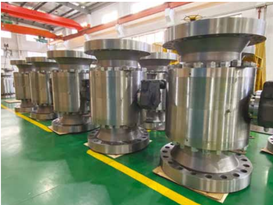
900lb valves during pressure testing.
