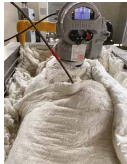
Actuated ball valve is being tested after 200 pcs operation at low temperature.
