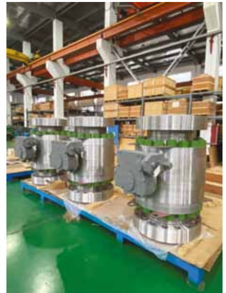
16" 1500lb valve during assembly.
