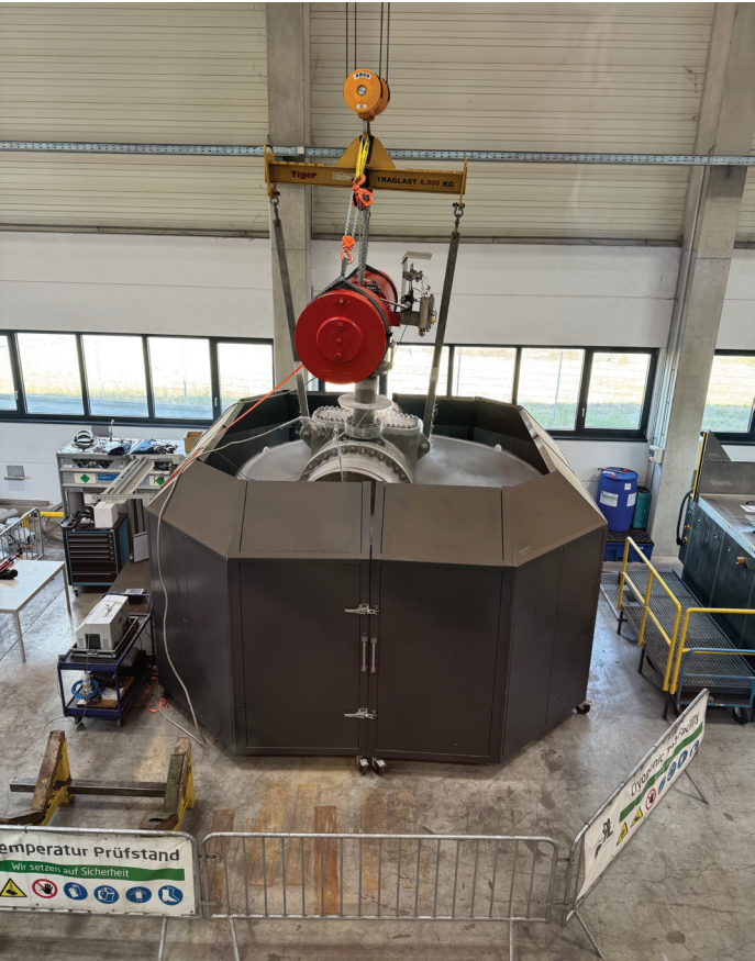
Cryogenic test of 42" 300# butterfly valve in OHL workshop.
