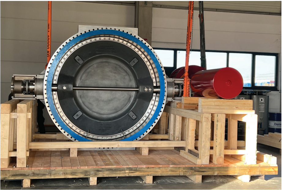
Triple offset butterfly valve 96" 300# for FCC at 760 degrees celsius.
