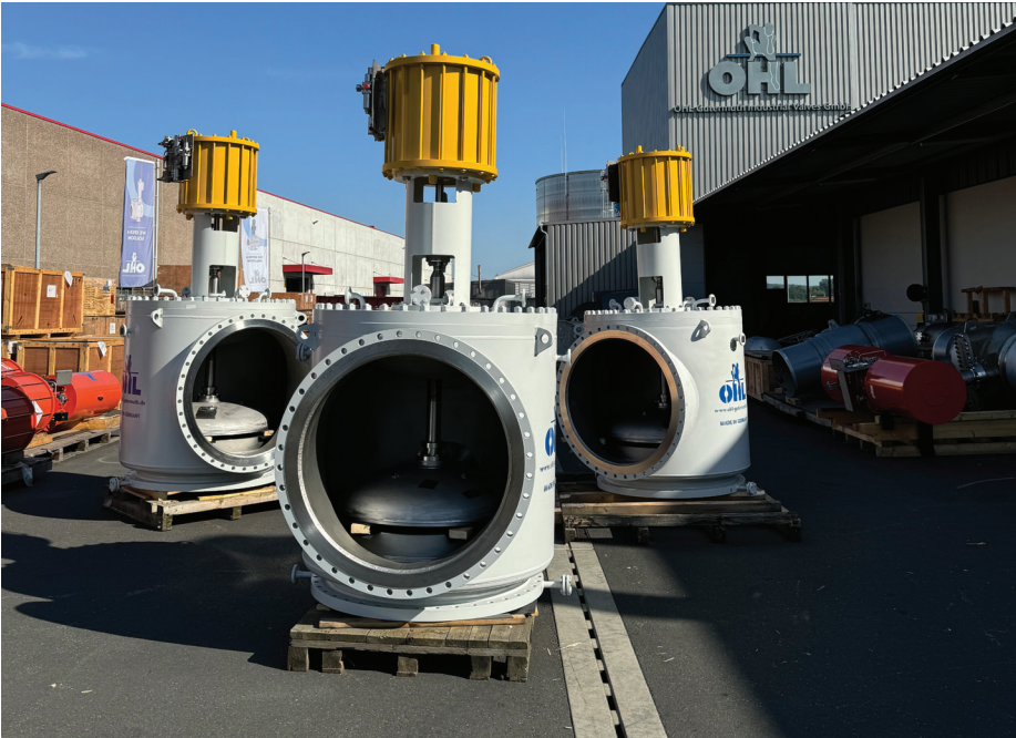
Reactor switching valves angle type for tail gas treatment.
