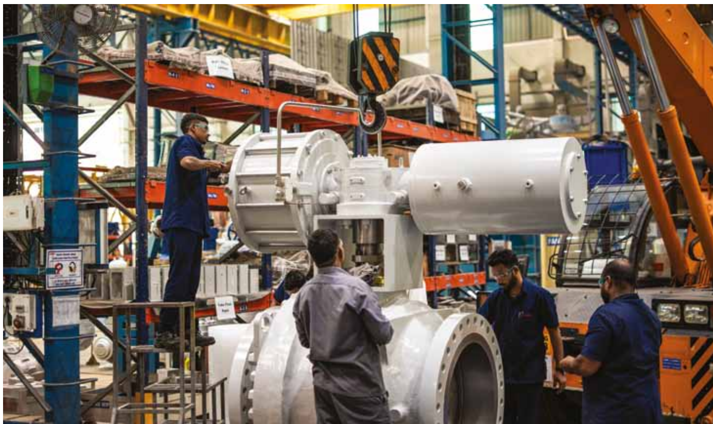
Final touches to a 30-inch metal seated ball valve
