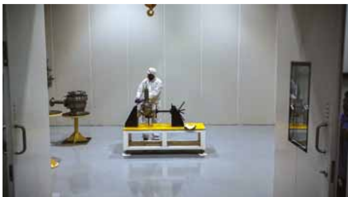
Oxygen service valve being assembled in clean room
