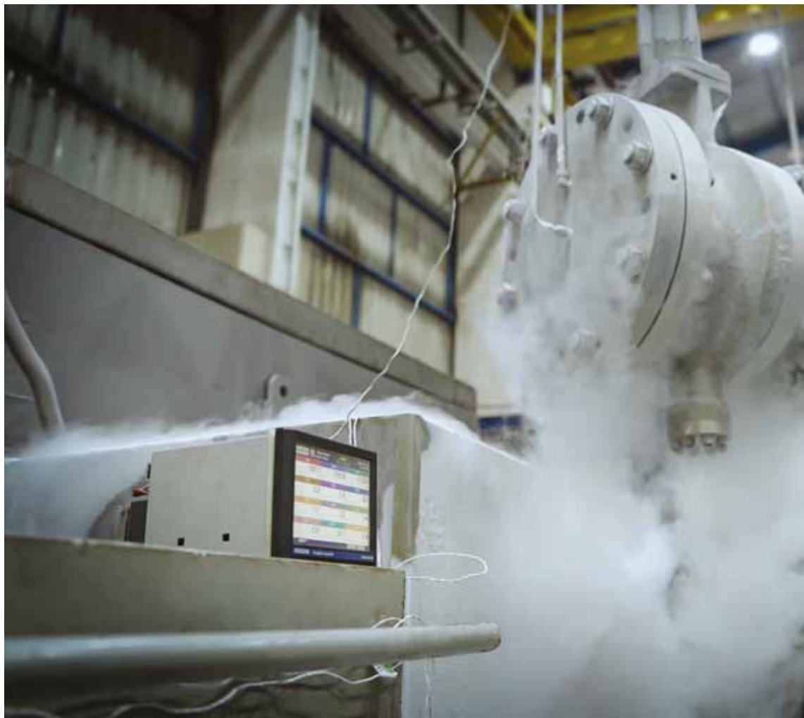
Cryo testing of control valve
