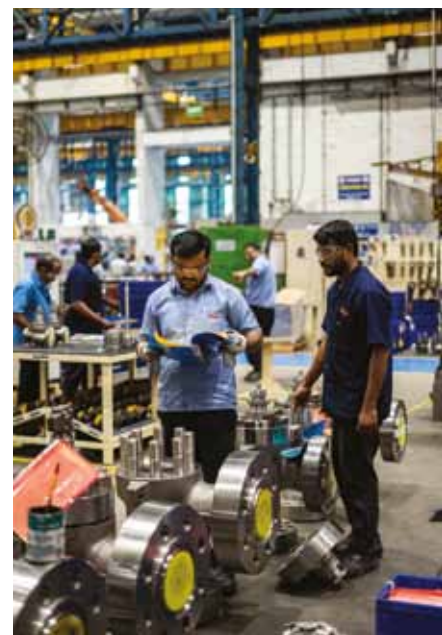
Valves under assembly
