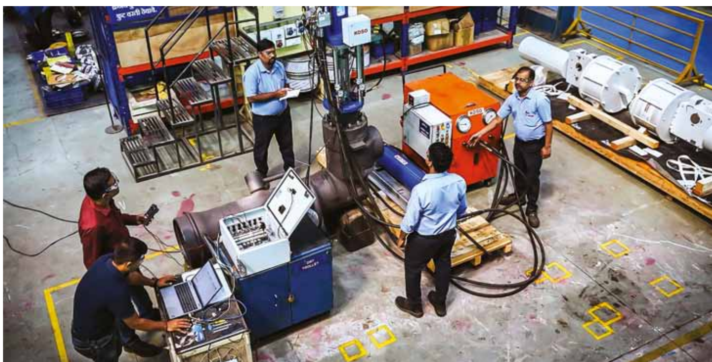
Testing of turbine bypass valve with Paladon Electrohydraulic Actuator
