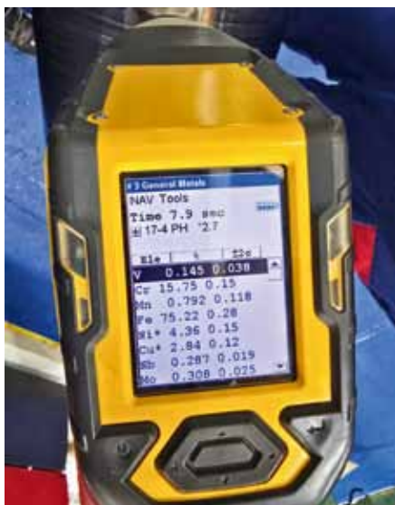
A Thermo Scientific Niton XL2 Gold Xray Gun is used to check chemical analysis.
