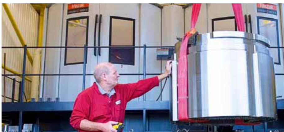
Mazak integrex 1850 carrying twin rotary tables of 2000mm diameter – 1500mm in the air. Depicting an aluminium extrusion press container manufactured from W.2344 (H13).
