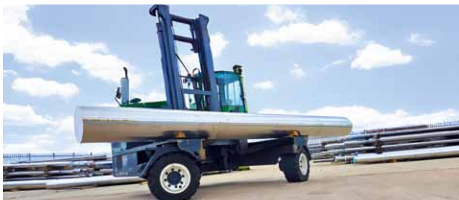
Combi lift with 15 tonne capacity lifting Ø535 x 8 meters long bar weighting 14.2 tonnes.
