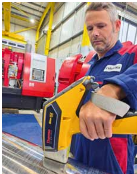
A Thermo Scientific Niton XL2 Gold Xray Gun is used to check chemical analysis.
