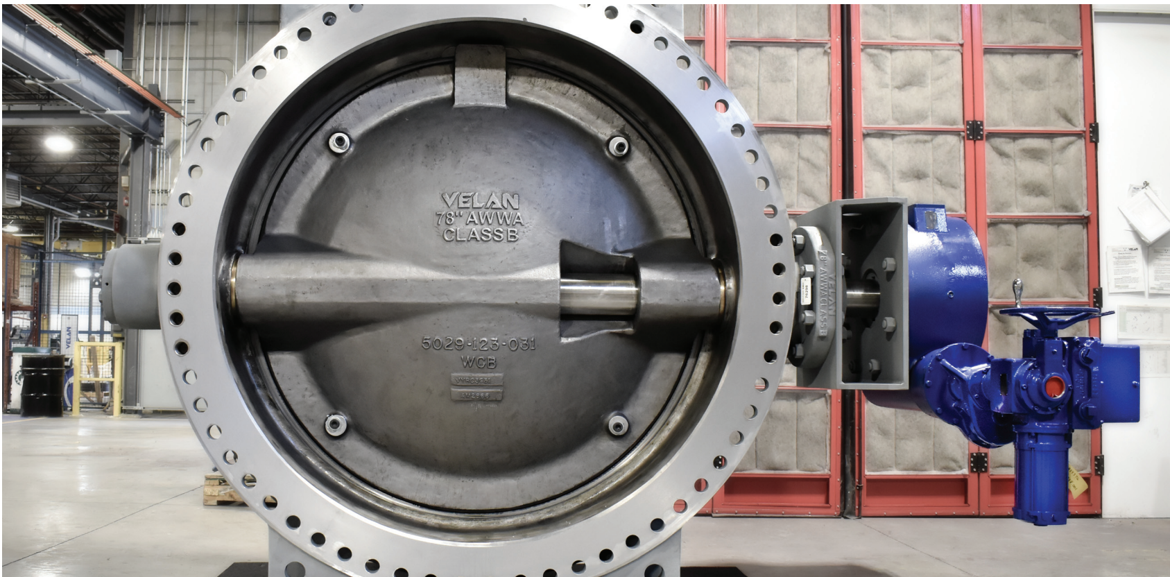
The impressive 78-inch Torqseal® triple-offset valve, the largest butterfly valve built at Velan.
