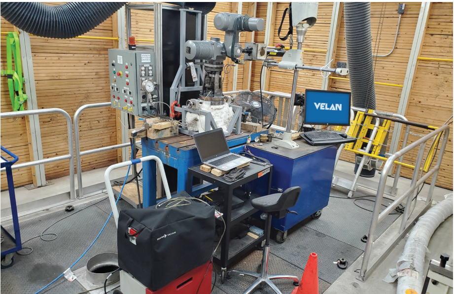
Fugitive emissions testing of a pressure seal valve in the 2020's.
