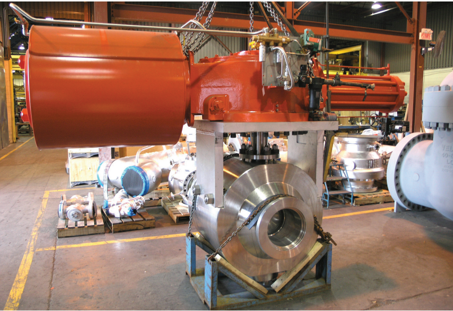
An 18-inch Securaseal® R-series severe service metal-seated ball valve headed to a refinery in the United States.
